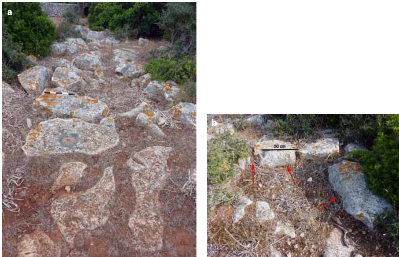
Figure 10. Quarrying beyond site limits. (a) Jointed limestone ca. 300 m SE of Building 2 (Fig. 2); meter scale is 50 cm. Such blocks are readily available for quarrying, as shown in (b), which is ca. 50 m away and shows the area in which some blocks have been removed (delineated by arrows).
