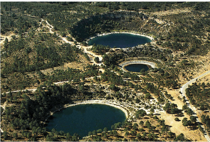
Lagunas de Cañada del Hoyo (Cuenca). Sinkholes or collapse dolines, formed in Cenomanian dolostones with an almost perfect circular shape and partially filled by ground water.
