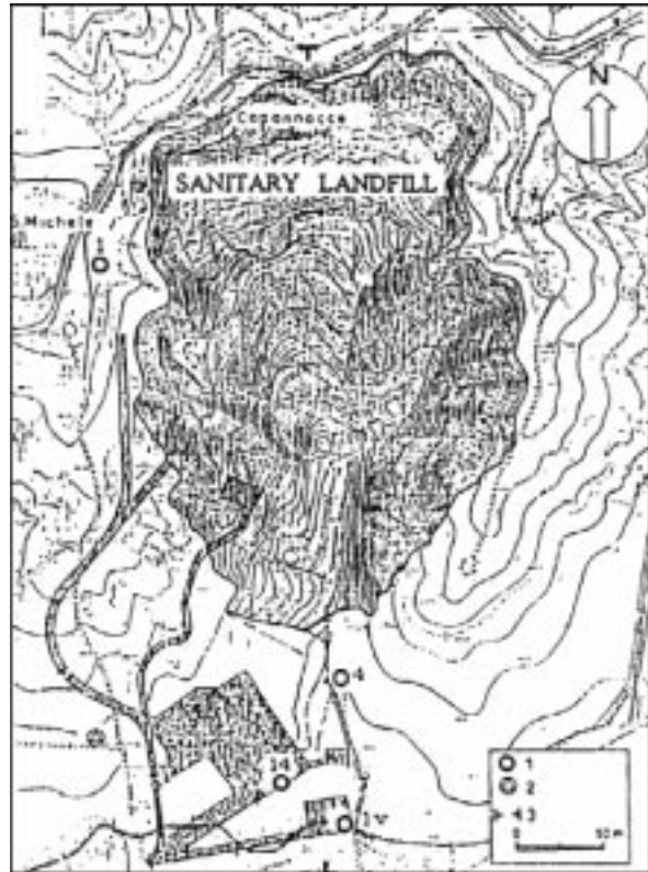
Fig. 11. Location of the landfill near Firenze, San Martino a Maiano. 1, borehole; 2, borehole equipped with piezometers at different depths; 3, trace of hydrogeological section of Fig. 12.
